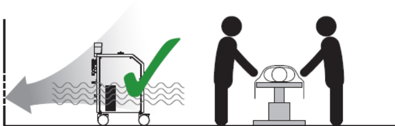
Fig. 4: Placing the heater-cooler in relation to the exhaust vent system
