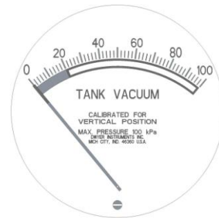
Figure 2) Tank Vacuum gauge with zero point and adjustment screw in the bottom part of the gauge
