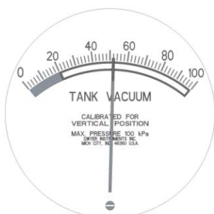
Figure 13) Tank Vacuum gauge with indicator in the acceptable area of operation and adjustment screw in the bottom part of the gauge
